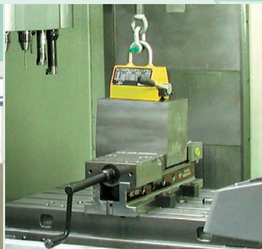
Application: Universal Permanent lift magnet SAV 531.01 mounted to shop crane
